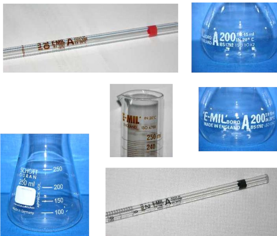
Figure 2-11. Illustrations of markings on volumetric glassware
