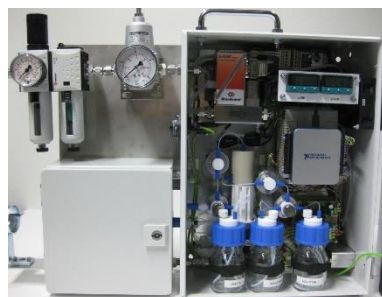
VTT's dynamic gas generator that uses liquid evaporation to generate wet reference gases;
